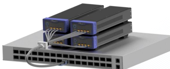
Figure 3 Switch Testing using 4 Pulsars.
